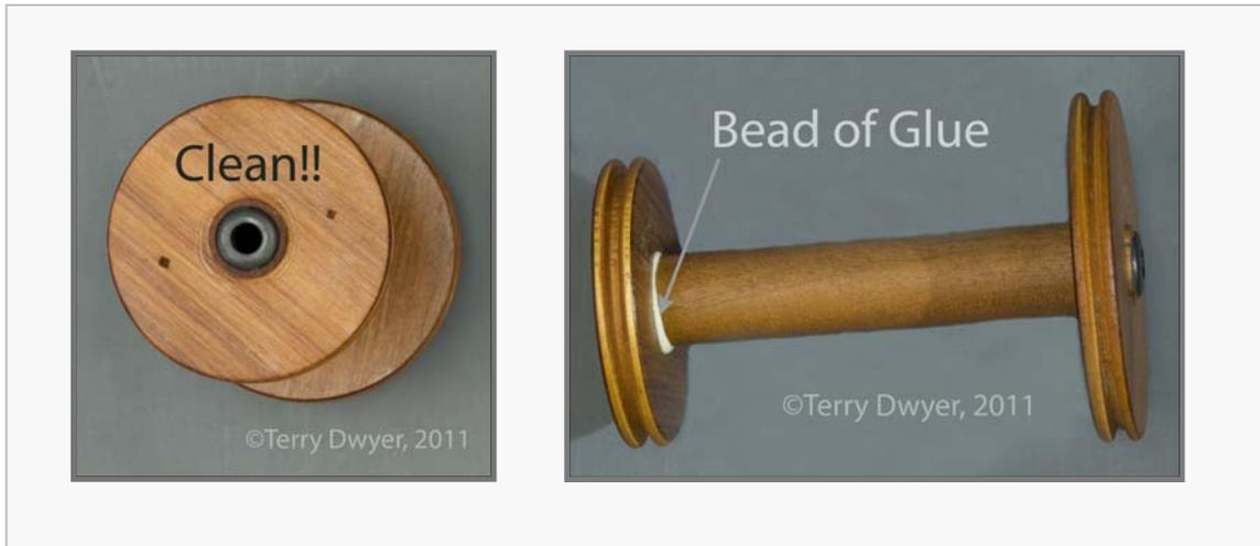
8. **»»» Belt-and-Suspenders Step «««** Here is an optional final step that will improve the repair (but it is not necessary). Tack a  $\frac{1}{2}$ " brad into the joint from the outside to push the axle firmly against the hole in the end piece and also create a key that will resist torque. Do your tacking on a platform that allows room for the axle to stick through.
